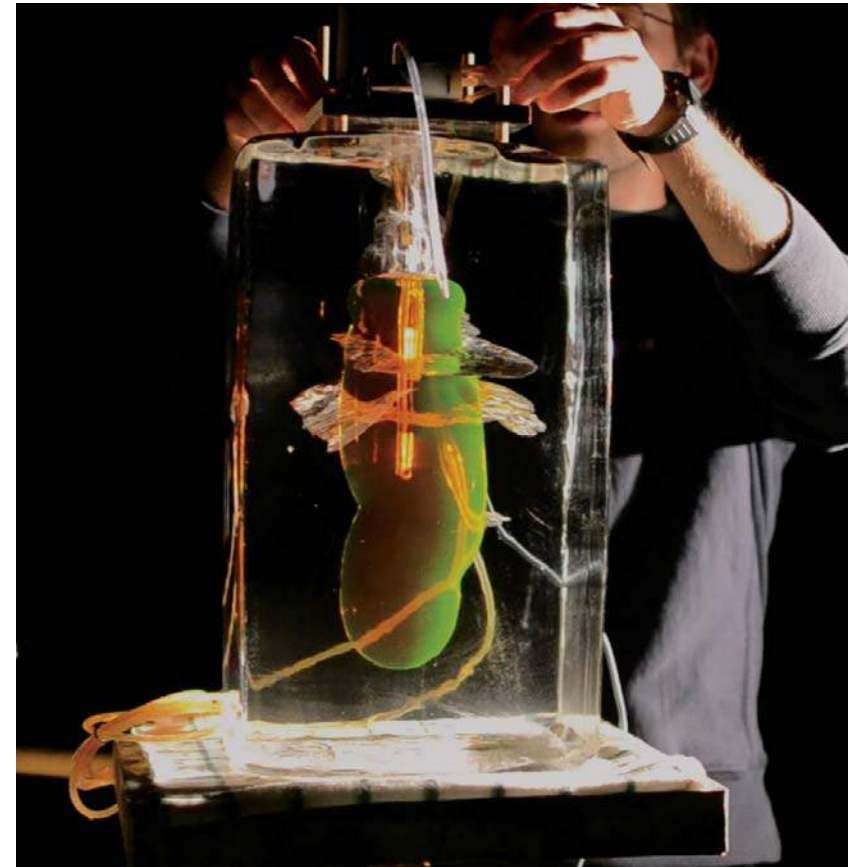
ESR 9 - VASILY SITNIKOV / ICE FORMED CONCRETE CASTING
